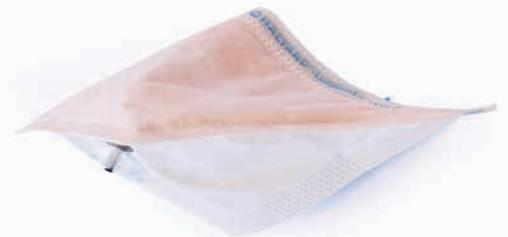
**Note:** Once a probe has been installed the respirator cannot be used for respiratory protection. As P2 and N95 respirators are single use, they must only be used to fit test one person. Respirators must be discarded after fit testing.
